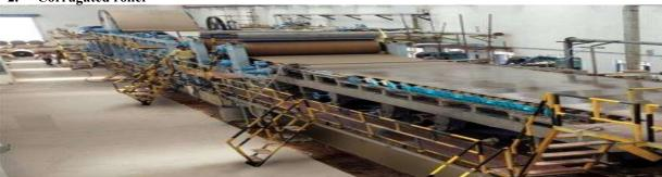
Corrugating roller is located at the base level and A liner is passed through pressurized rollers via dry steam another liner is passed through corrugated roller which gives the shape of corrugation to the middle liner and thus, corrugated waves are produced. 5 ply online corrugation machine with double profile flute for the combination of B and C flute carton which is as per the international norms and standards is used for the same. There are different hot plates and the adhesive for
