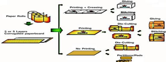
Printing is performed on corrugated box blanks that have been formed, scored and cut by a corrugator. The box blanks are subsequently cut or Die-cut into specific shapes for further forming into finished boxes. Printing Machine require 2 main operator and 6 helper in order to match the speed of the production
