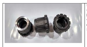
**Ultra Cast Iron Bearing Sleeve** used in Front Loading washing machines of four different sizes, said to be the heart of every washing machine, is machined by us within 10 microns bore accuracy, 30 microns concentricity between both bearing bores and surface finish of 1.6uRa.
