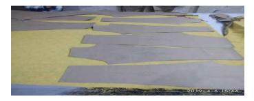
Step 4 Cutting of the Fabric according to the Marking/Pattern
