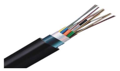
This cable is designed in such a way to withstanding the mechanical stresses applied to overhead lines due to environmental factors such as wind and ice. It must also be capable of handling electrical faults on the transmission line by providing a path to ground without damaging the sensitive optical fibers inside the cable.
